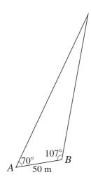
Some walkers see a tower, T, in the distance and want to know how far away it is. They take a bearing from a point A and then walk for 50 m in a straight line before taking another bearing from a point B. They find that angle TAB is 70° and angle TBA is 107° (see diagram).
